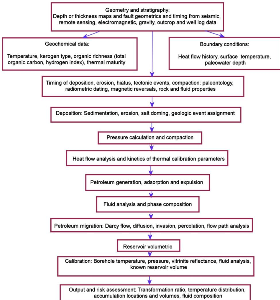
**Figure 2.** Workflow chart illustrating the steps of BPSM (Basin and Petroleum System Modelling) [Al-Hajeri *et al.*, 2009].
