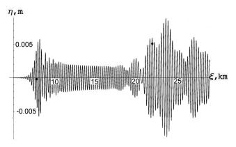
**Figure 6.** Elevation  $\eta$  at y = 3 km,  $M = 0.4 < M_0$ .
