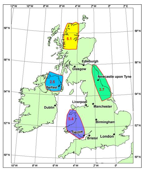
**Figure 5.** Regional model of the GUZs obtained using GEO-GIS. The numbers inside each zone indicate the predicted maximum earthquake magnitude within that zone.
