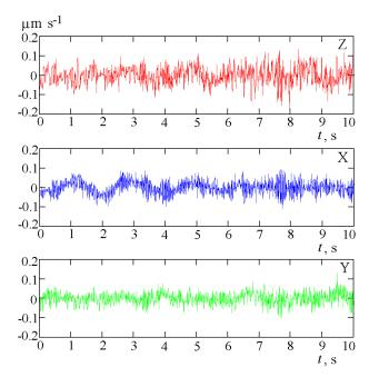
Figure 4. Velocigrams of microseismic background at 8 h, 50 min, September 02, 2000. Astrophysical Neutrino Observatory, (Z) vertical, (X) N-S horizontal, and (Y) W-E horizontal.
