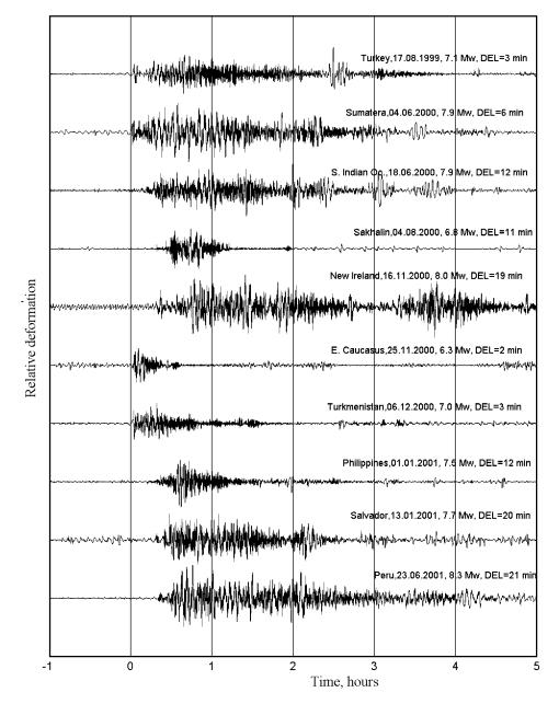
Figure 8. Observed deformations, plotted using the period of data discretization equal to 2 seconds [Sobisevich et al., 2001, 2002a]
