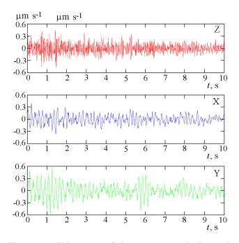
Figure 3. Velocigrams of the microseismic background recorded by the Astrophysical Observatory at 2 h, 00 min, September 04, 2000: (Z) vertical, (X) N-S horizontal, and (Y) W-E horizontal.
