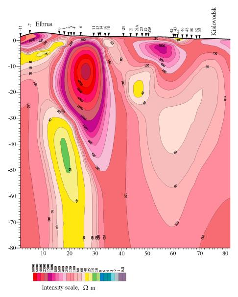
Figure 11. The resistivity section representing the interpretation of the data obtained by the magnetotelluric sounding performed along the North Elbrus profile. The horizontal axis is the distance along the profile in km, the vertical axis being the depth in km. The left edge of the section is the south, the right one being the north. The equal resistivity contour lines are plotted after [Arbuzkin et al., 2002].
