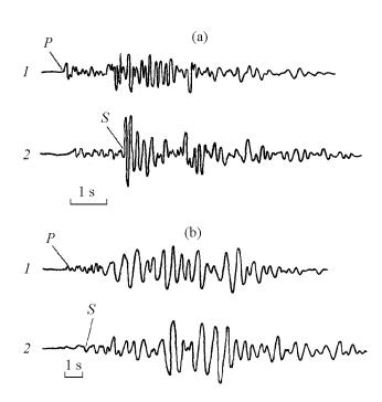
Figure 2. Seismic records of local earthquakes in the North Caucasus region: (1) Caucasus mineral water area, (2) Elbrus Cone area: (a) a vertical component, (b) a horizontal component [*Khitarov et al.*, 1984].
