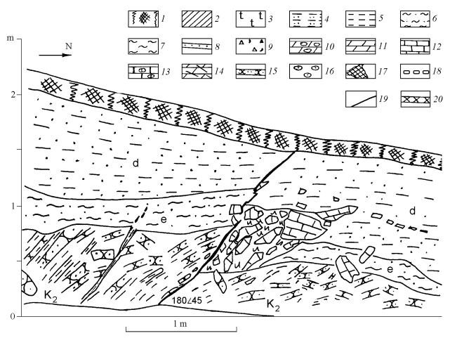
Figure 5. Sketch drawing of western wall of a trench across the active Kuznetsovsky fault (composed by E. A. Rogozhin). In the center, a debris wedge filled with limestone fragments is clearly seen.
