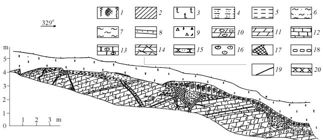
**Figure 8.** Sketch drawing of southwestern wall of a trench across the Drovyanoi active fault (composed by E. A. Rogozhin, A. N. Ovsyuchenko, E. A. Ushanova, A. V. Marakhanov, and N. A. Dvoretskaya). In the center, a small scarp on the base of the modern anthropogenic ("technogenic") layer above a fault branch is clearly seen.
