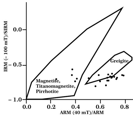
**Figure 6.** Biplot diagram of dependence of IRM (–100 mT)/SIRM from ARM(40 mT)/ARM.
