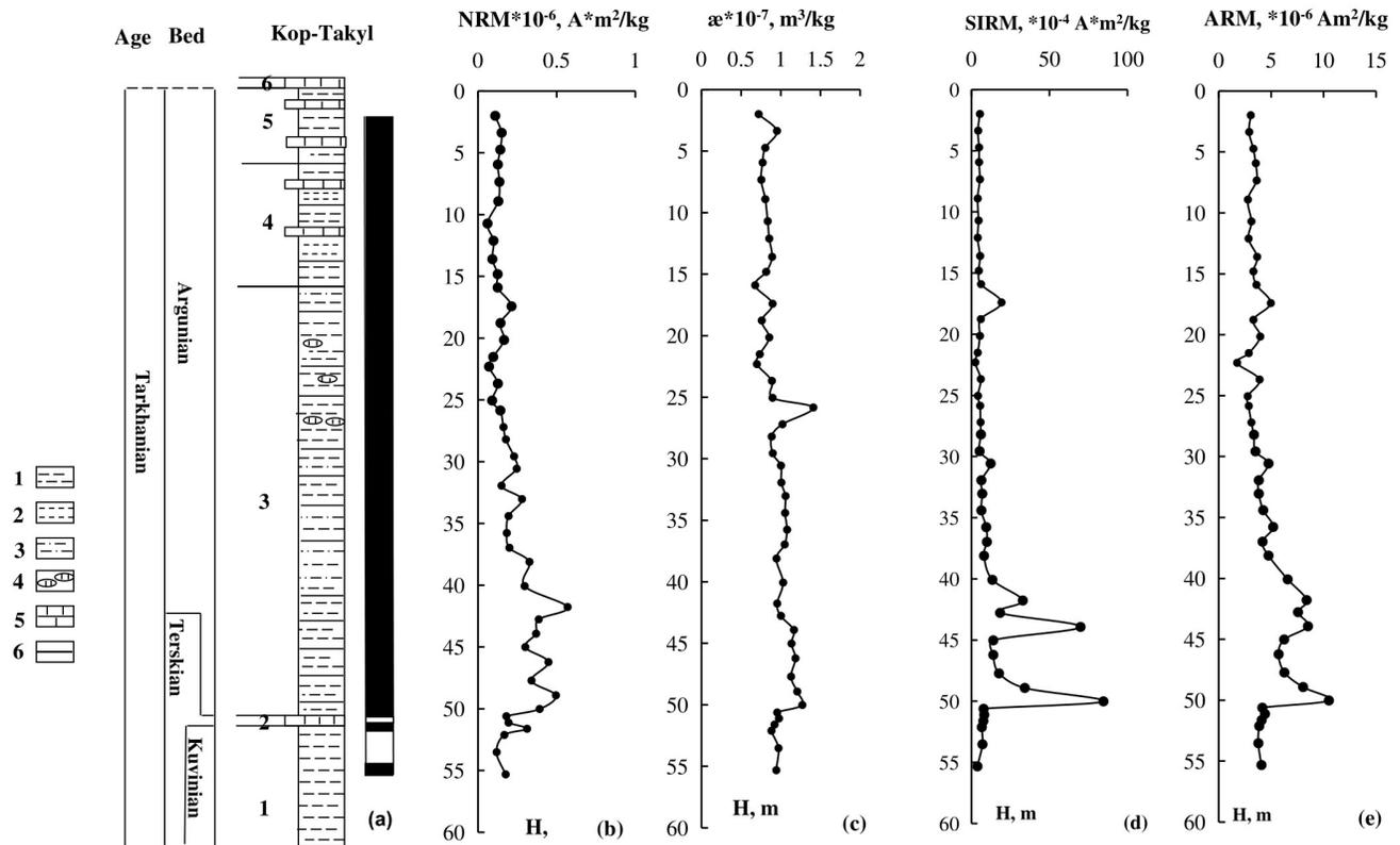
**Figure 2.** Lithological column of the Kop-Takyl section (a). Legend: 1 – clay, 2 – calcareous clay, 3 – clay with thin sandy layers, 4 – carbonate nodules, 5 – carbonate layers, 6 – layer boundaries. Variations curves of the magnetic characteristics versus section depth  $H$ : natural remanent magnetization NRM (b), mass magnetic susceptibility  $\chi$  – (c), saturation isothermal remanent magnetization SIRM – (d), anhysteretic remanent magnetization ARM – (e).
