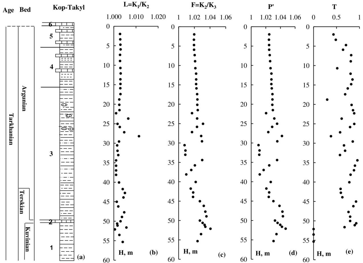
**Figure 10.** Lithological column of the Kop-Takyl section – (a). Dependence of AMS parameters versus section depth H: L – (b), F – (c),  $P'$  – (d), T – (e).
