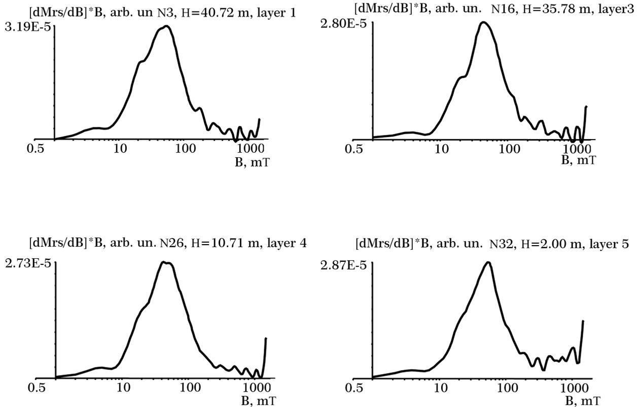
**Figure 7.** Coercive spectra of isothermal remanent magnetization.
