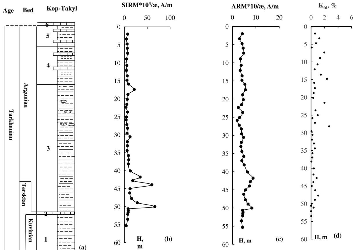
**Figure 9.** Lithological column of the Kop-Takyl section – (a). Curves of changes in grain size ratios versus section depth  $H$ : SIRM/ $\alpha$  – (b), ARM/ $\alpha$  – (c), frequency-dependent parameter  $K_{fd} = (K_{lf} - K_{hf}) * 100\% / K_{hf}$  – (d).
