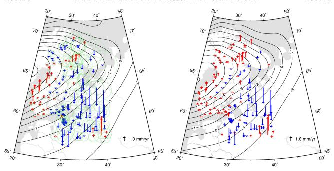
**Figure 4.** The arrows give the residuals of our result w.r.t. the model of Glacial Isostatic Adjustment (GIA) by *Lambeck et al.* [1998]. The isolines were digitized from the paper. The −2 mm/year isoline is our own extrapolation Most of our TG rates were used in the construction of the GIA model. The green circles show our formal 1-sigma error estimates.
