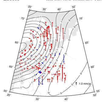
**Figure 9.** The residuals are relative to the hybrid model NKG2016LU (version KG2016LU\_lev relative to the geoid). We have subtracted 1.3 mm/yr to account for the rise in MSL (1892–1991).
