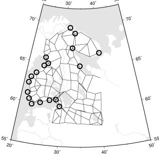
Figure 2. The total levelling network and the tide gauges (open circles). In this paper only the Baltic tide gauge rates are used. For the purposes of the adjustment, the a-priori standard error of 0.5 mm/year was assigned to them. The presentation of the network is schematic, straight lines connect the nodal points.
