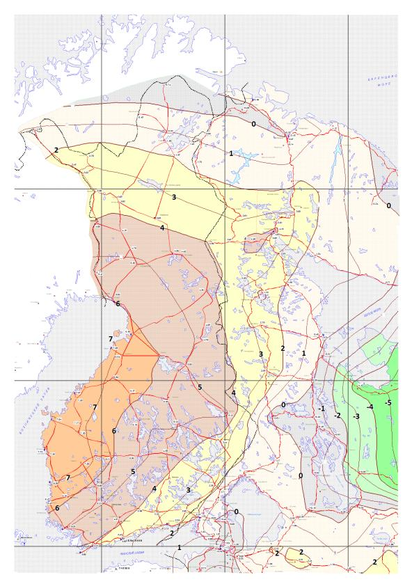
**Figure 3.** Map of the velocities of the vertical recent crustal movements of the region compiled by TsNIIGAiK. Interval between isolines is 1 mm/yr.
