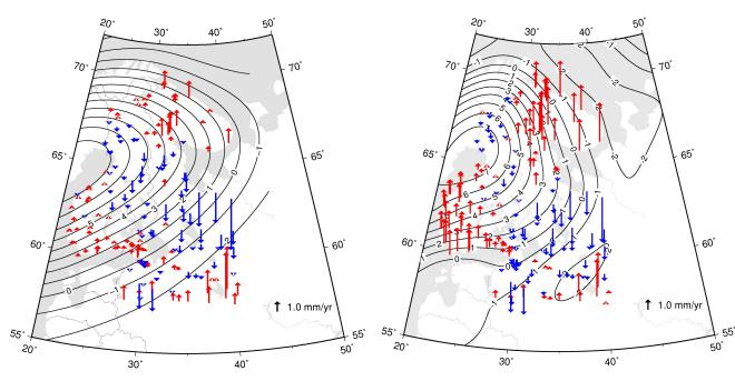
Figure 6. The same rates but residuals are now relative to the GIA model by Milne et al. (2001). The "absolute" GIA rates relative to the Earth's center of mass were converted to rates relative to MSL assuming a geoid rise of 6% of the absolute rates and a MSL rise of 1.3 mm/yr (1892–1991).
