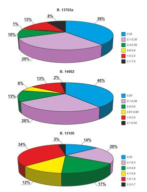
Figure 5. Model distribution of classes (%) of contents (ppm) of Au in ore and wallrocks intervals of boreholes of Myutenbay deposit (the region of deep boreholes of MS-2 and MS-3). Borehole, 15100.
