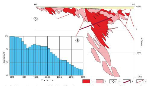
Figure 6. A schematic section and depth of development of the central part of Muruntau deposit (A) and dynamics of gold content change in the process ore in time (B). According to [Sitenkov et al., 2005]. 1 – rich ore columns with ore content > 0.8; 2 – low-grade ore bodies with ore content < 0.3; 3 – gold-bearing quartz veins; 4 – dyke of a plagioporphyry; 5 – faults.
