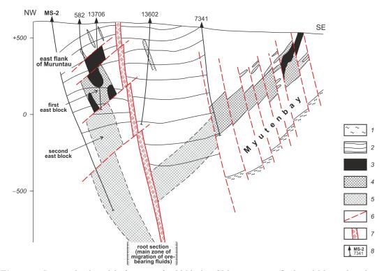
**Figure 4.** Longitudinal model of a ratio of gold blocks of Muruntau east flank and Myutenbay deposit (GE line 136). According to [*Obraztsov*, 2001]. 1 – carbon-micaceous schist; 2 – interstratified micaceousquartz schist and metaaleurolites; 3 – balance ore; 4 – outbalance ore; 5 – lean and underexplored ore zones; 6 – faults; 7 – tectonic zone; 8 – boreholes.
