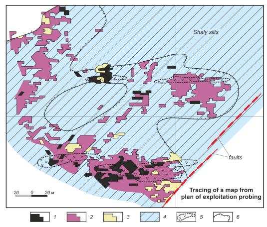
**Figure 3.** Nature of distribution of gold on Muruntau deposit in an ore zone (detailed exploration), according to operational exploration [*Obraztsov*, 1998]: Ores: 1 – bucking, 2 – run of mine; 3 – barren rock; 4 – interstratified shaly silts; 5 – zone of quartz vein; 6 – borders of ore zone according to data of detailed exploration.
