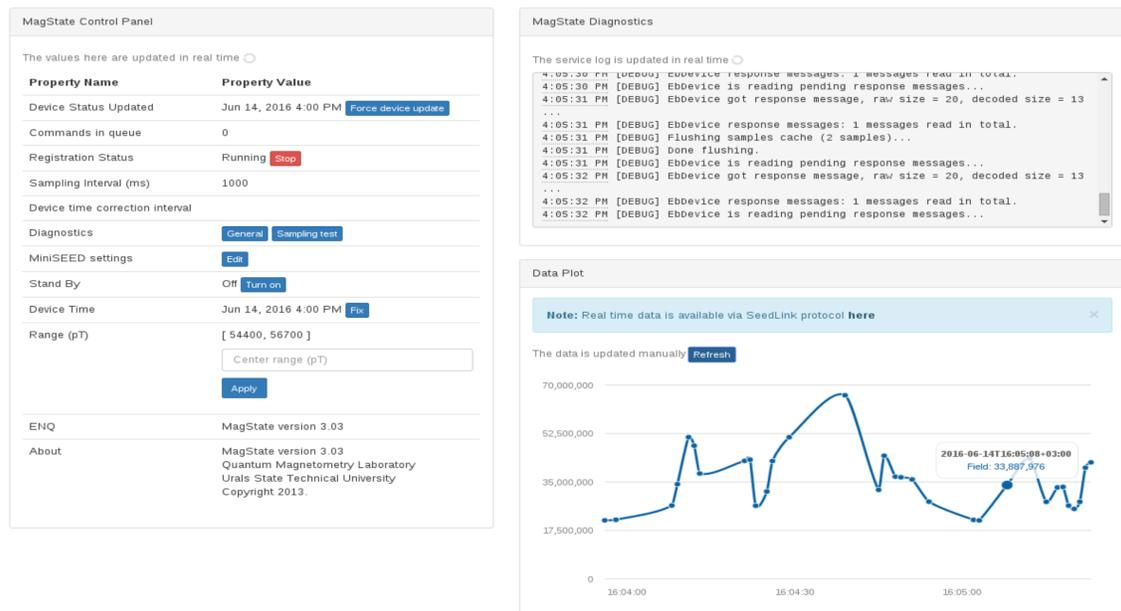
**Figure 2.** Web user interface is a flexible yet very accessible way to manage the system. The operator can use virtually any web-aware device to set up and monitor the system. Underlying REST API also allows any kind of automated management and monitoring as well as further integration with large-scale software.
