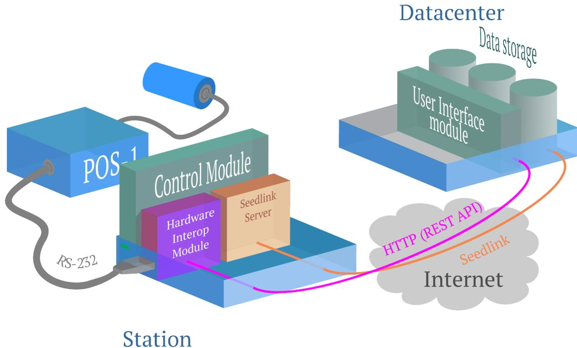
**Figure 1.** POS-1 measures geomagnetic field and transfers the results to Hardware Interop Module – the adapter program. The module handles the data further to the Seedlink server that is available to both the Datacenter and local/remote clients. Control Module component manages all station-run services. User Interface component manages the Control Module component via web.
