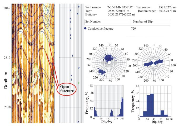
Figure 6. Open fracture on the image log, Stereonet rose diagrams and histograms.
