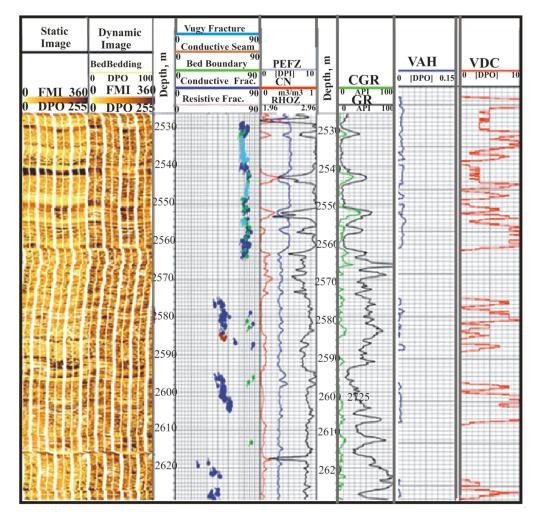
**Figure 4.** Image log and petrophysical logs in the understudy well. Abbreviations are: FMI: formation micro image, PEFZ: photoelectric factor, CN: compensate neutron, RHOZ: density log, CGR: compensate gamma ray, GR: gamma ray, VAH: apparent hydrolic fracture aperture, VDC: fracture density.
