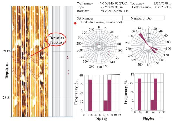
Figure 7. Resistive fractures on the image log, Stereonet rose diagrams and histograms.
