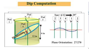
**Figure 2.** Schematic illustration of fracture plane intersecting a cylindrical borehole, indicating how the strike and dip of the fracture is interpreted from televiewer log images of the intersection between the fracture plane and the borehole wall.
