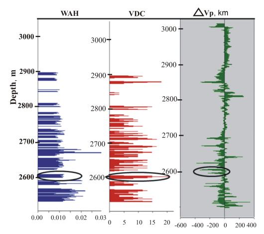
Figure 12. The plot shows more negative values of VDC in zones with high fracture aperture and so high fracture density velocity deviation. VAH controlled deviation of VDL values.
