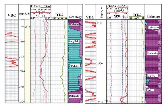
Figure 11. The plot indicates the effect of mineralogy on the fracture density. Abbreviations: NPHI: neutron porosity, DT-2: sonic log.
