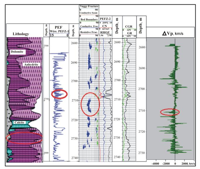
Figure 5. Comparison between lithology, image log and VDL showing negative values of VDL in zone with thin bedded dolomite layer. Abbreviations: PEF: photo electric factor,  $\Delta Vp$ : variation of velocity deviation.
