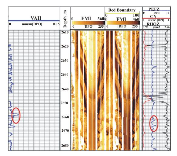
Figure 10. Comparison between the zone responses having fractures with higher aperture (VAH) and petrophysical log (PEF). 8 of 11
