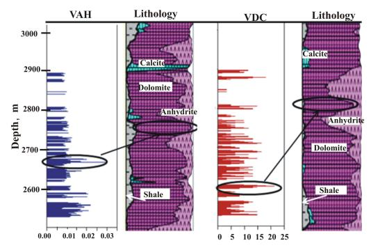
Figure 9. Role of lithology on fracture density (VDC) and fracture aperture (VAH).
