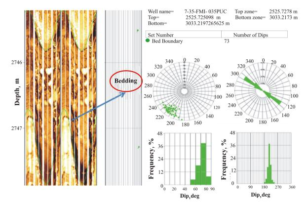
Figure 8. Bedding on the image log, stereonet rose diagrams and histograms.
