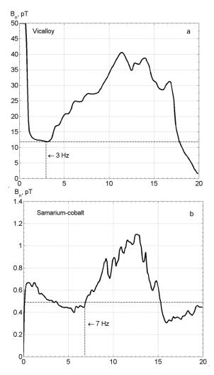
**Figure 4.** The detailed spectra of signals at the output of the vicalloy based (a) and samarium-cobalt based (b) variometers in the frequency range from 1 to 20 Hz.
