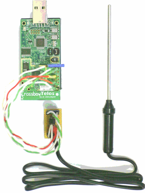
Figure 2. TelosB platform with attached thermocouple and infra-sound microphone.
