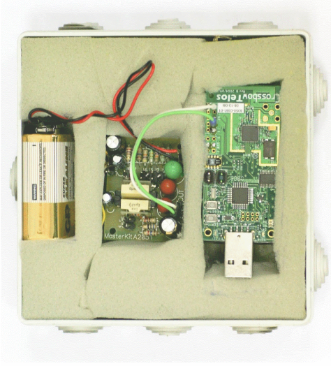
Figure 2. TelosB platform with attached thermocouple and infra-sound microphone.
