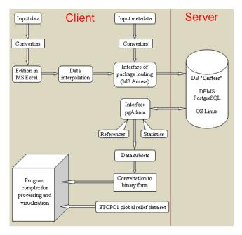
**Figure 1.** The scheme of the system of storage, processing and visualization of drifter data.
