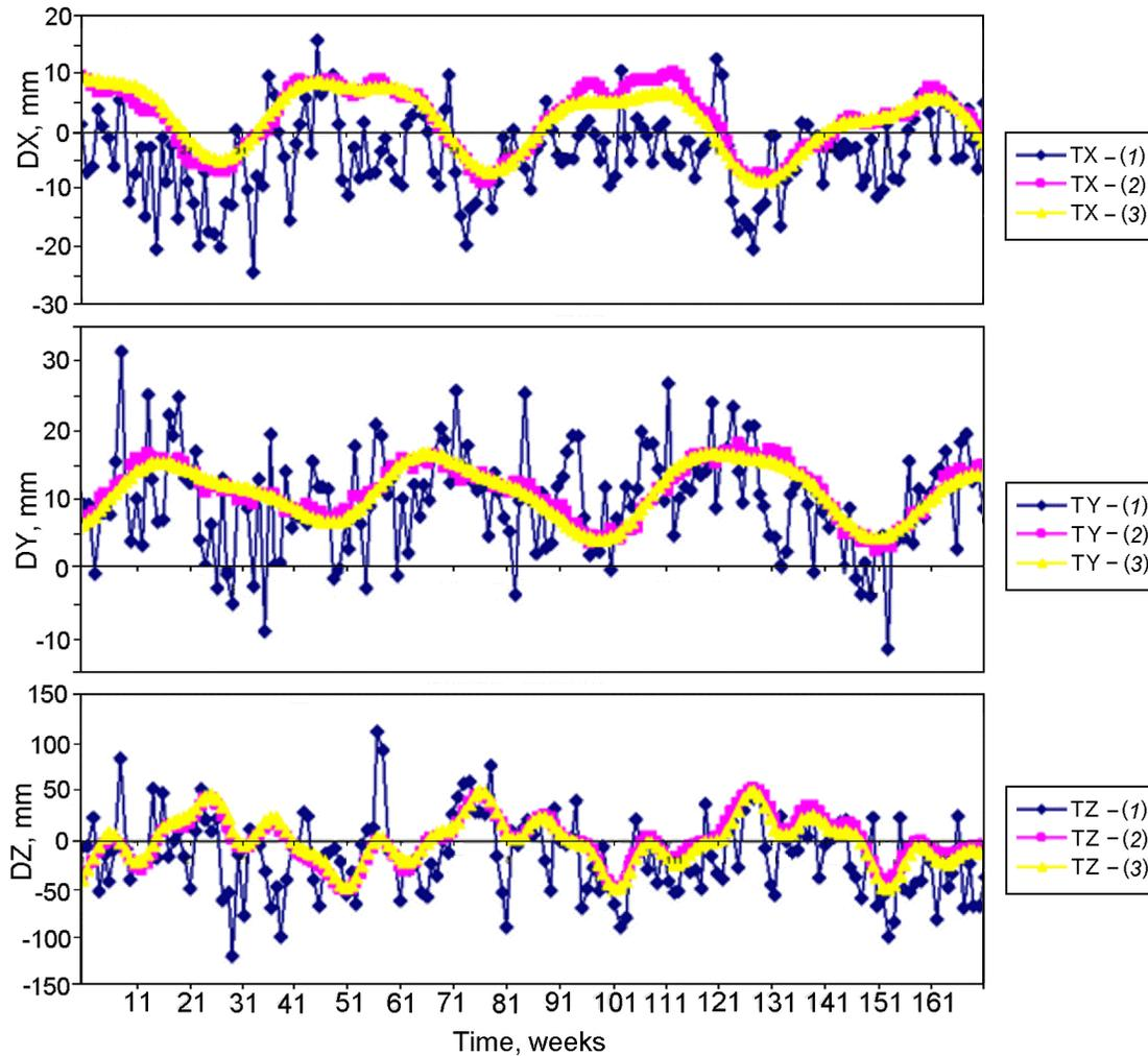
**Figure 1.** Diagrams of geocenter positions, estimated by the truncated (1), complete (2) mathematical models and by the real DORIS observations (3).
