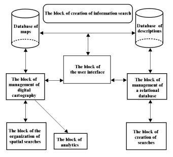
Figure 2. Principle functions of GIS.
