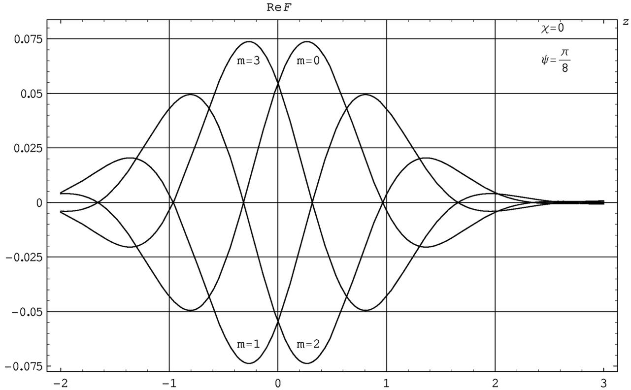
**Figure 6.** The profile metamorphosis implied by the Maslov (Morse) index: function  $\text{Re}[e^{-\frac{i\pi\mathbf{m}_j}{2}} F(z, \psi)]$  for  $V(y)$  determined by (6) where  $V_0 = 1$  m,  $a_1 = a_2 = 0$ ,  $b_1 = 1$ ,  $b_2 = 2$ ,  $\chi = 0$  corresponding to the Maslov (Morse) indices  $m = 0, 1, 2, 3$ .
