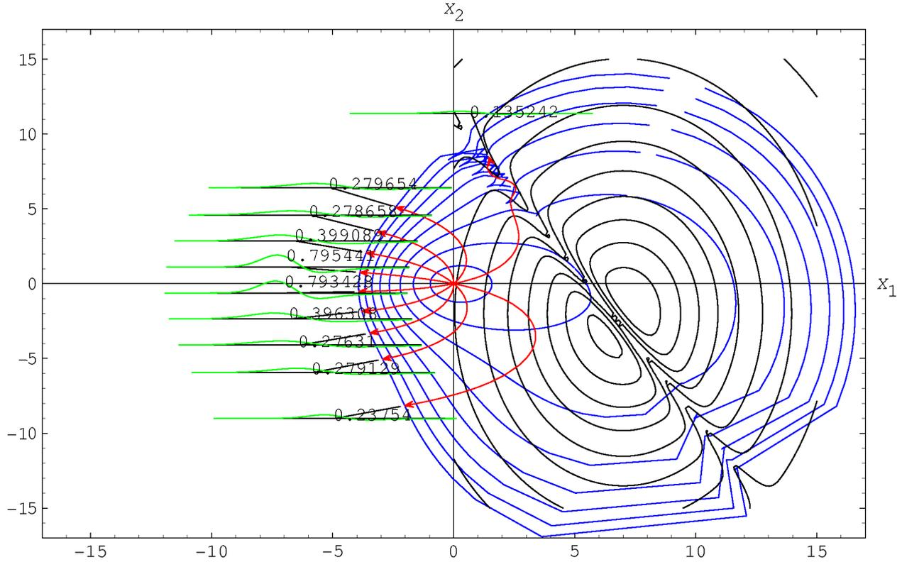
**Figure 3.** Wave fronts, rays and profiles in the case of the basin with non-uniform depth (see text).  $V(y)$  is determined by (6) where  $V_0 = 1$  m,  $a_1 = 0$ ,  $a_2 = 2$ ,  $b_1 = 1$ ,  $b_2 = 0.25$ ,  $\psi = 0$ ,  $\chi = 0$ .
