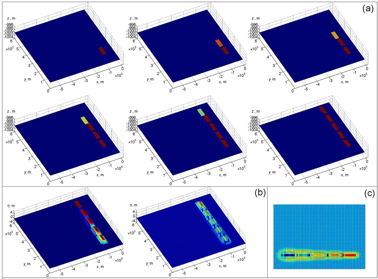
**Figure 5.** The example of successive block motion in earthquake source (a); The example of generation of surface water wave by seismic source: (b) for two time moments, (c) the view from upper point.
