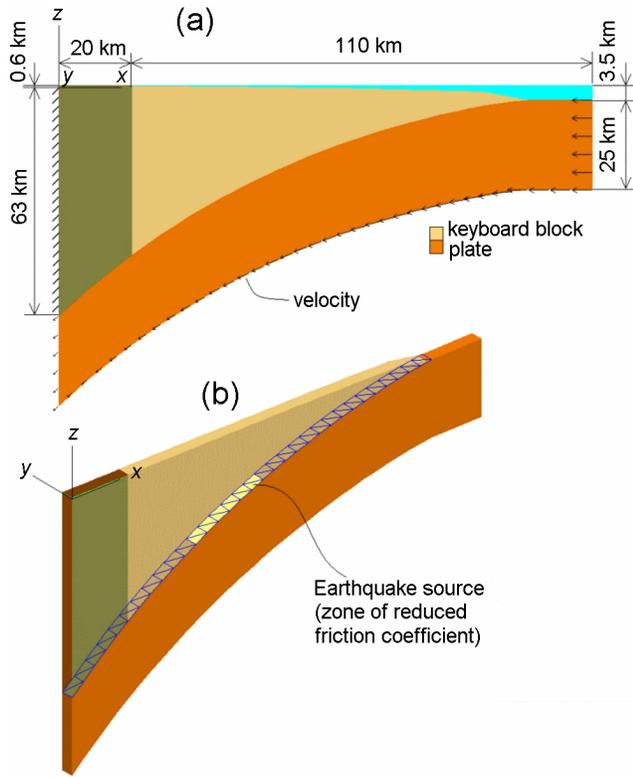
**Figure 14.** Sketch of the computational model subduction zone.
