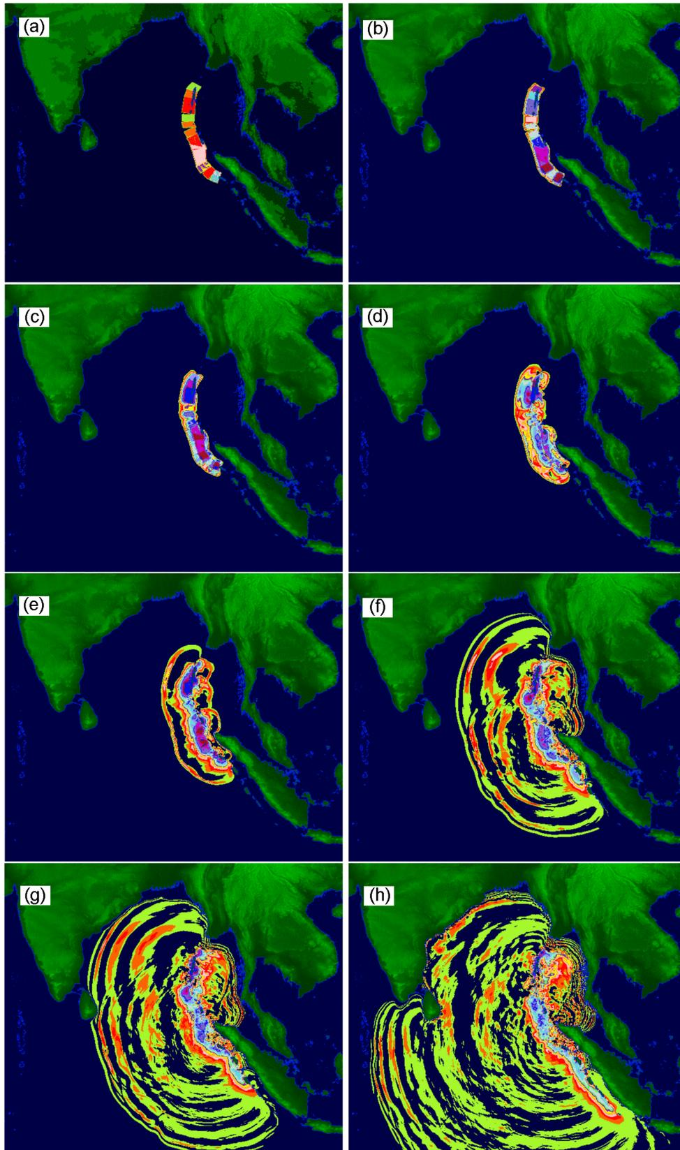
**Figure 22.** Generation and propagation of tsunami waves in the basin of the Indian Ocean for the seismic source comprising 14 blocks for the time moments: a –  $t=20''$ , b –  $t=2'20''$ , c –  $t=4'50''$ , d –  $t=16'30''$ , e –  $t=33'10''$ , f –  $t=1h50'$ , g –  $t=2h30'$ , h –  $t=4h18'$ .
