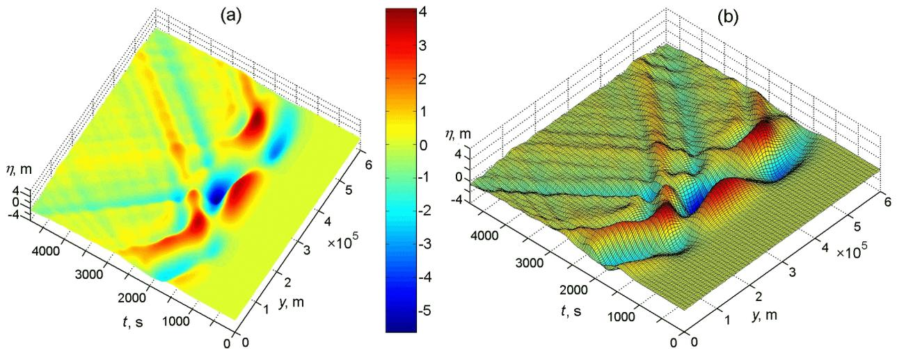
**Figure 10.** Space-time picture distribution of maximum wave run-up along shoreline for tsunami source consisting of keyboard blocks of the different size (Figure 6b); successive motion of blocks in the source: a) 2D simulation; b) 3D simulation.
