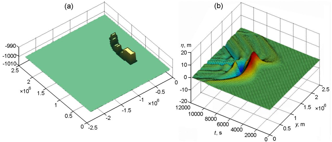
**Figure 13.** Modelling of the source of tsunamigenic earthquake 26 December, 2004 by motion of eight keyboard blocks moving along the subduction zone one after another from south to north (a); space-time picture of the moving shoreline(b). Maximum run-up is equal to  $R_{max} = 11$  m, run-down  $R_{min} = 10$  m.
