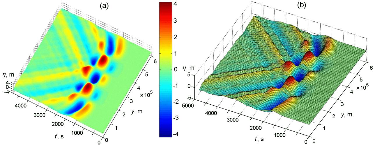
**Figure 9.** Space-time picture distribution of maximum wave run-up along shoreline for tsunami source consisting of keyboard blocks of the same size (Figure 6a); successive motion of blocks in the source: a) 2D simulation; b) 3D simulation.
