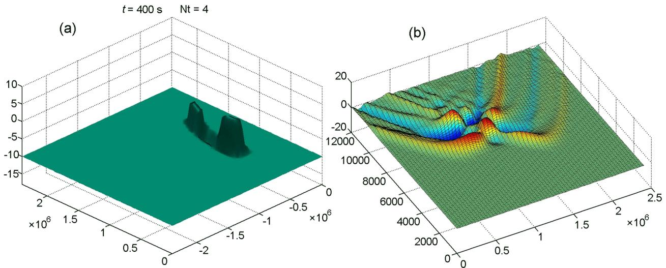
**Figure 12.** Modelling of the source of tsunamigenic earthquake 26 December 2004 by motion of three keyboard blocks rising along the subduction zone one after another from south to the north (a); space-time picture of the moving shoreline(b). Maximum run-up is equal to  $R_{max} = 9.5$  m, run-down  $R_{min} = 7.5$  m.
