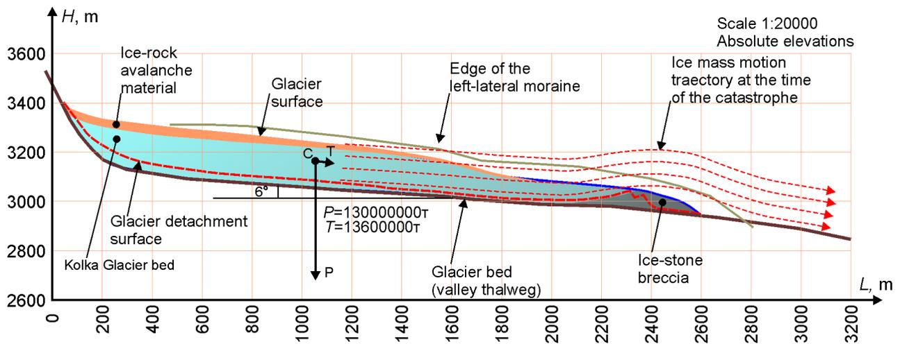
Figure 20. The reconstruction of the longitudinal vertical section of the Kolka Glacier.
