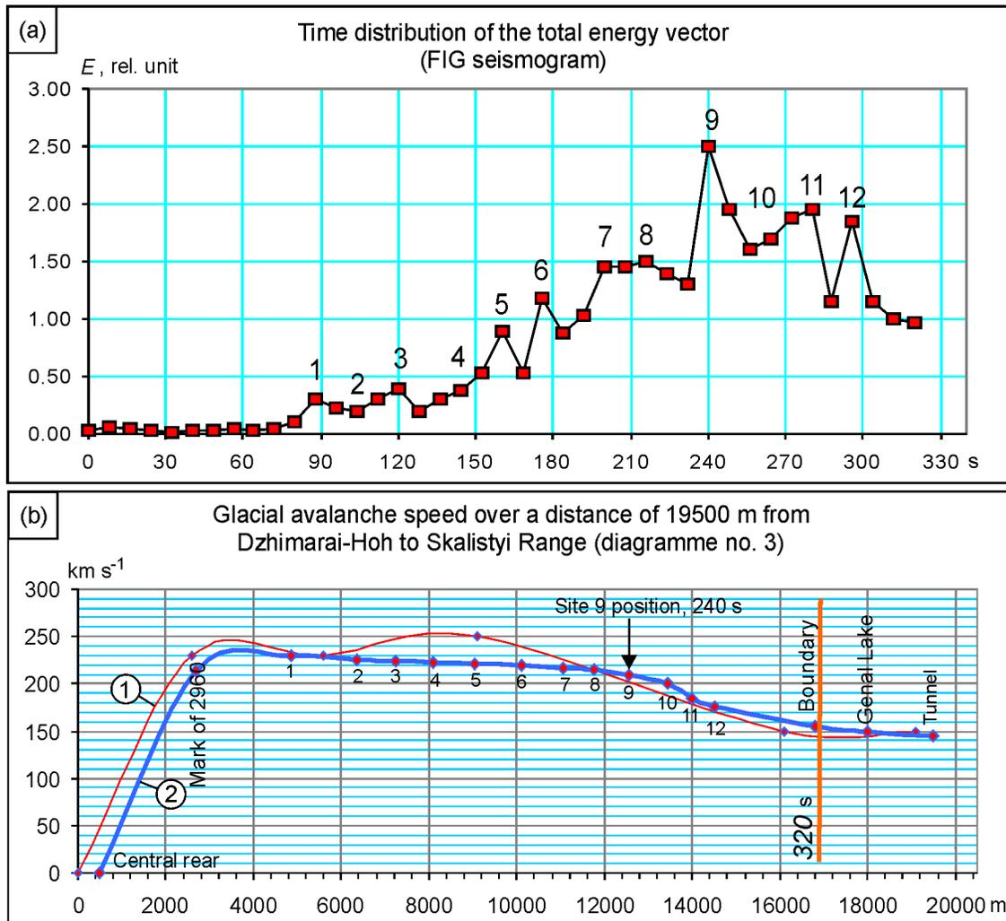
Figure 19. The diagrams illustrating some of the parameters of the Kolka Glacier caving. Shown in Diagram B are (1) the curve of the avalanche velocities, calculated from the geometry of the trace left by the avalanche and (2) the curve of velocity distribution, satisfying the seismic records.
