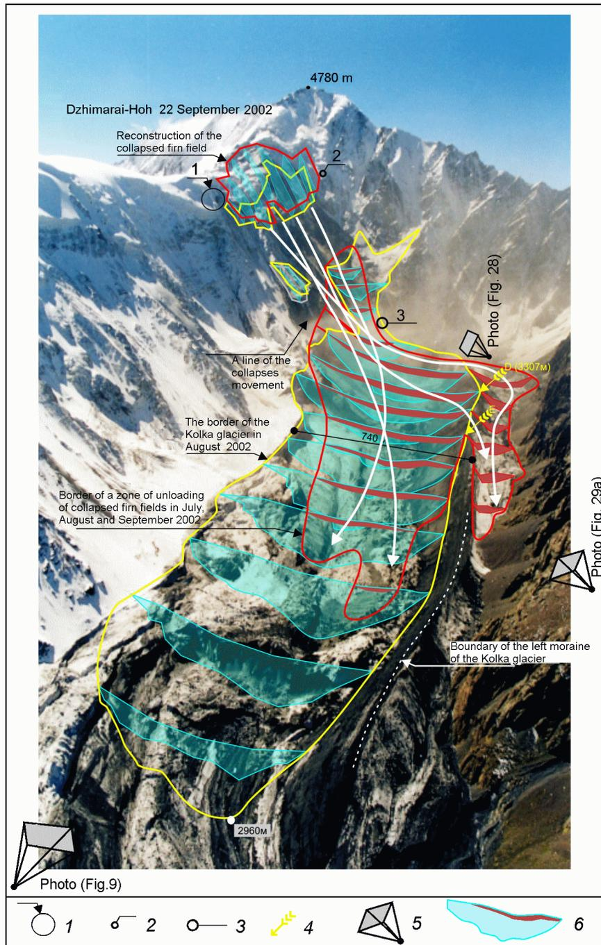
**Figure 13.** Focus area of glacial catastrophe. 1-3 – identification areas and points; 4 – a line of the collapses movement; 5 – points of shooting for the photos; 6 – reconstructed sections of the Kolka glacier body with a designation of thickness of the collapse-rocky material.
