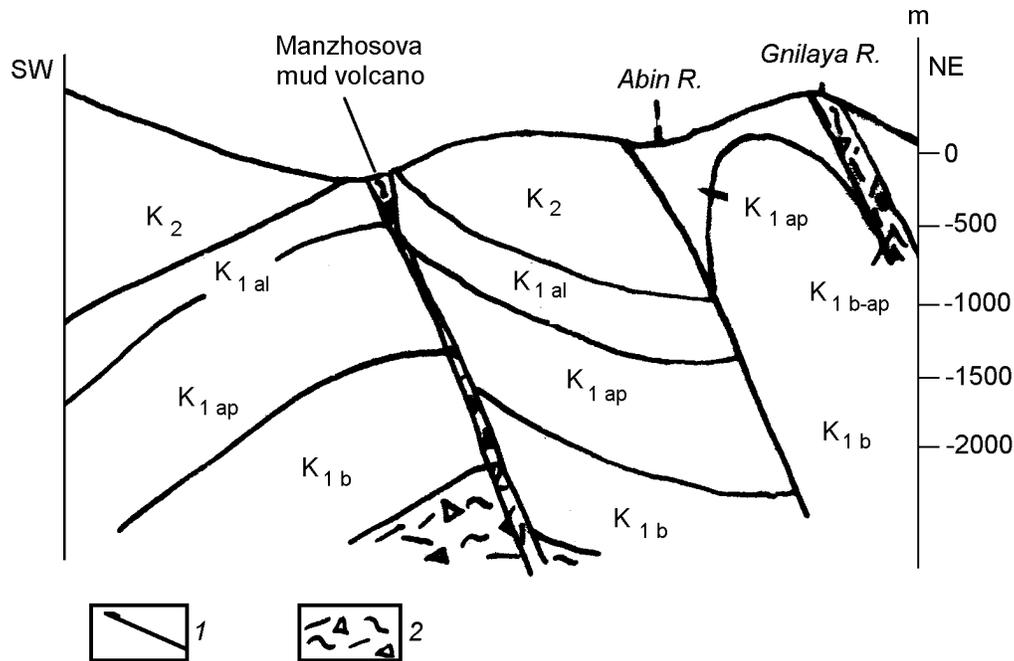
**Figure 4.** Geological section across Manzhosova mud volcano. 1 – geological boundaries; 2 – unconsolidated clayey matter with limestone fragments.
