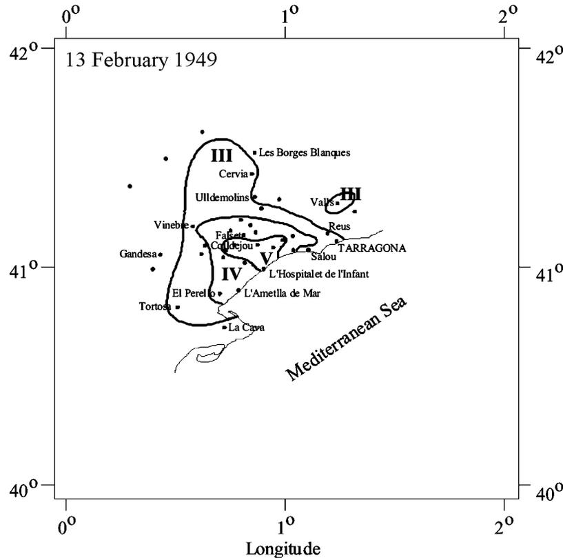
**Figure 3.** Isoseismal map for the 13 February, 1949 earthquake [Mézcuá, 1982]; source Fontseré [1951].
