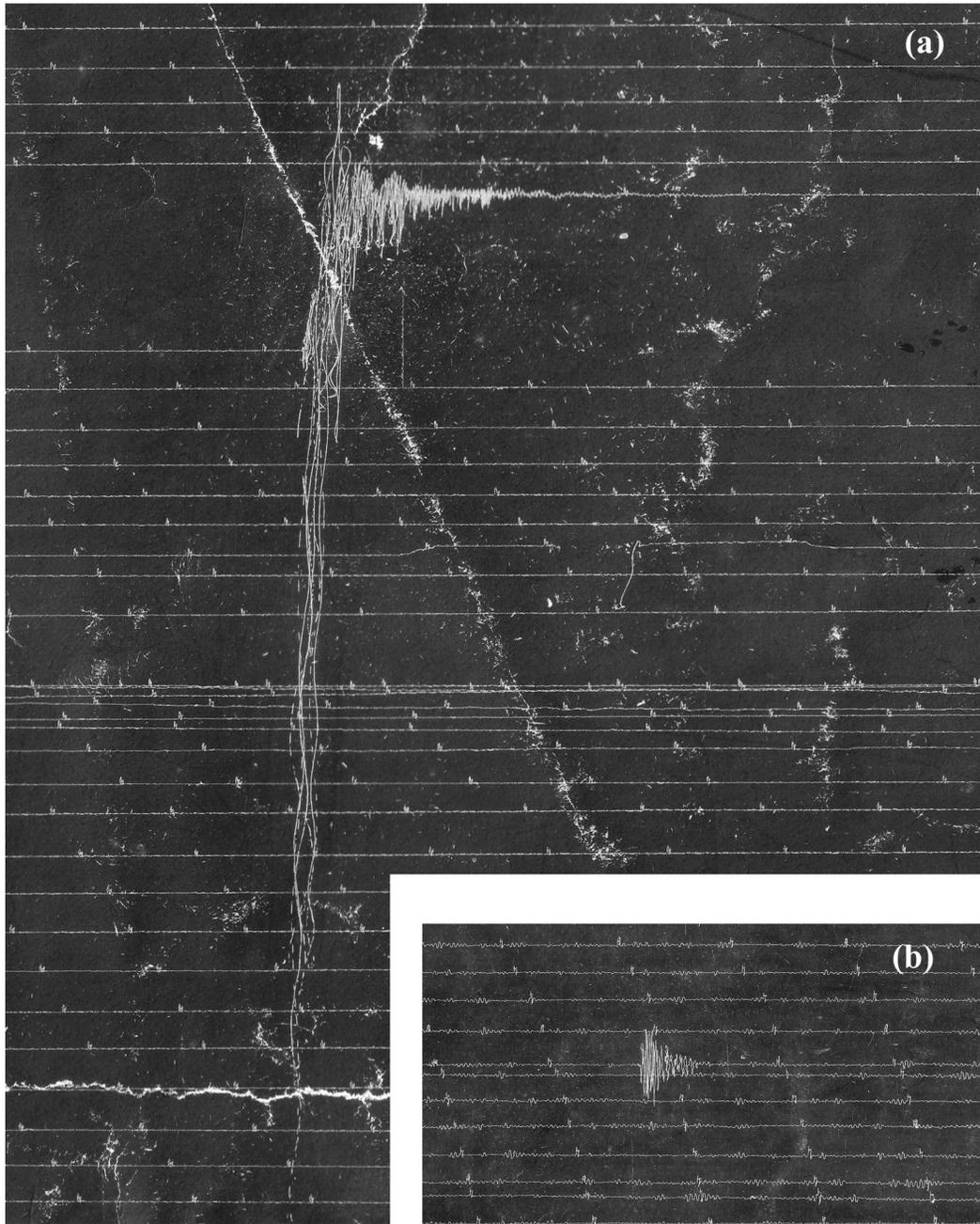
**Figure 6.** Example of the (a) 2 June, 1930 and (b) 13 February, 1949 earthquake records at EBR Observatory (N-S component of the Mainka Seismograph). Both seismograms are plotted at the same scale.
