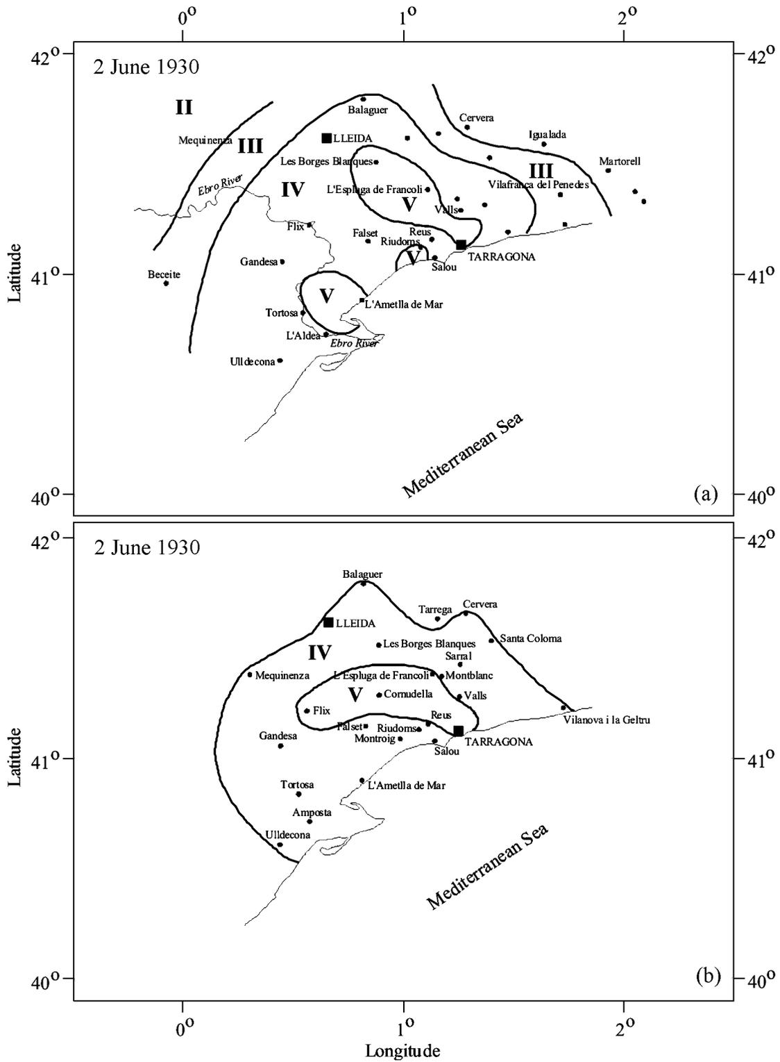
**Figure 2.** Two versions of the isoseismal maps for the 2 June, 1930 earthquake [Mézcu, 1982], (a) source SSIS and (b) source Fontseré [1940].
