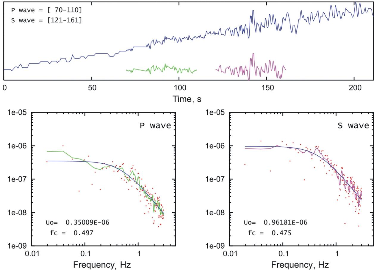
**Figure 5.** Example of one digitized signal recorded by the NE-SW component Wiechert seismograph at Toledo Observatory. The best fits for the seismic moment calculation for P and S waves are also shown.
