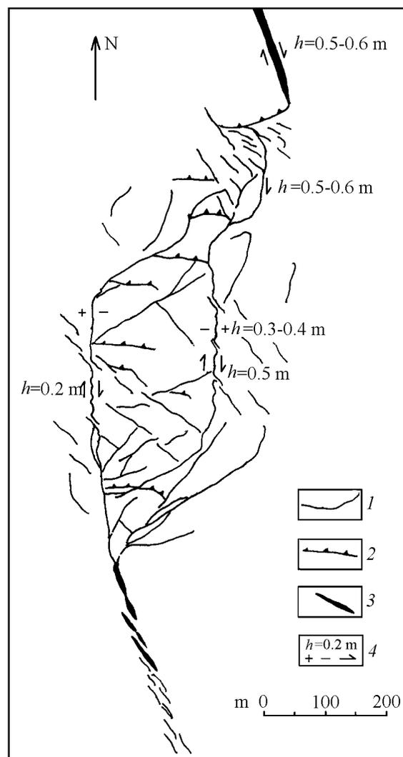
**Figure 2.** The structure of a seismic rupture in the area of the Chagan R. and Elangash R. watershed. (1) Closed fissures and cracks, (2) compression ridges, (3) seismic trenches, (4) amplitude and direction of offset.
