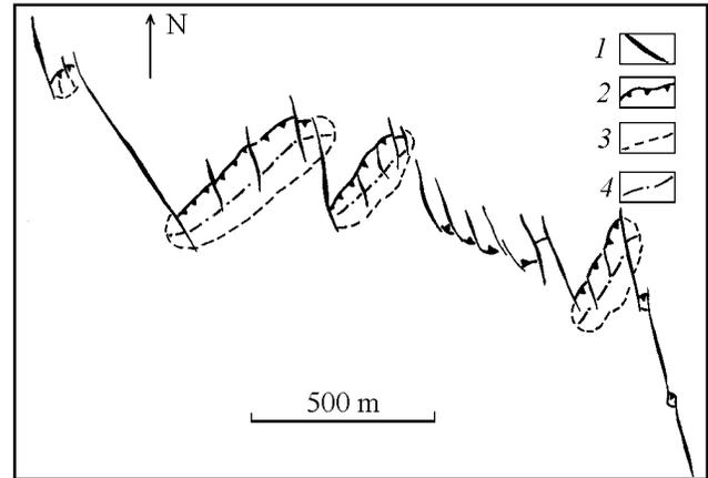
**Figure 7.** The structure of a seismic fault in the area of the watershed between the Taldura and Kuskunnur rivers. (1) seismic trench or open fracture; (2) dextral pressure ridges thrust scarp; (3) pressure ridge outline; (4) dextral pressure ridges axis.
