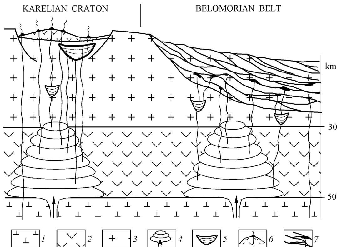
**Figure 6.** Structure of magmatic systems in the large Baltic SHMS Province as a function of tectonic conditions. (1) Ancient lithospheric mantle; (2) ancient lower crust; (3) ancient sialic crust; (4) paths of magma batches ascending through the crust by the mechanism of zone refinement; (5) transitional chambers (layered intrusions); (6) volcanosedimentary deposits in rift-related structures; (7) zone of tectonic flow into the Belomorian Mobile Belt.
