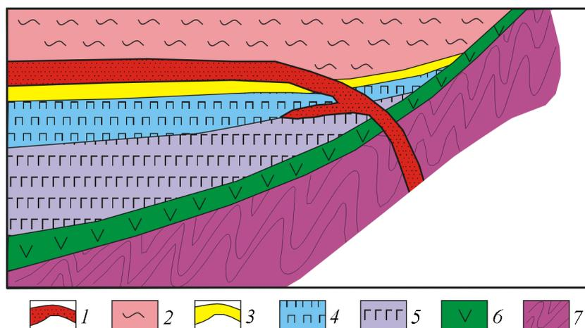
**Figure 5.** Replenishment of fresh magma into a crystallizing intrusive chamber (with reference to the “Sopcha ore bed” in the Monchegorsk Pluton). (1) Fresh magma; (2) evolved magma in the intrusive chamber; (3) zone of crystallization; (4) orthopyroxene cumulate; (5) peridotite cumulate; (6) lower marginal zone; (7) Archean wall rocks.
