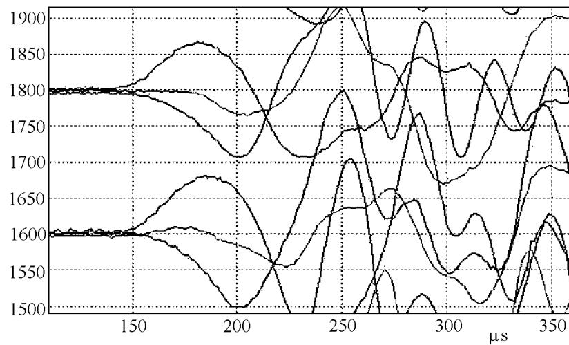
**Figure 2.** A fragment of the wave pattern obtained with the help of the 3-D piezoelectric transducers.
