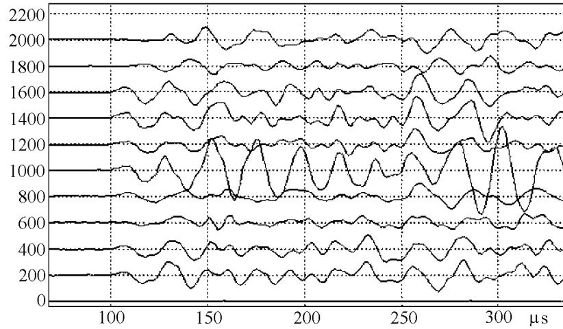
**Figure 6.** The wave pattern obtained on the metallic cylinder. Coordinate  $Y$  (direction across the axis of the cylinder tangent to the surface).
