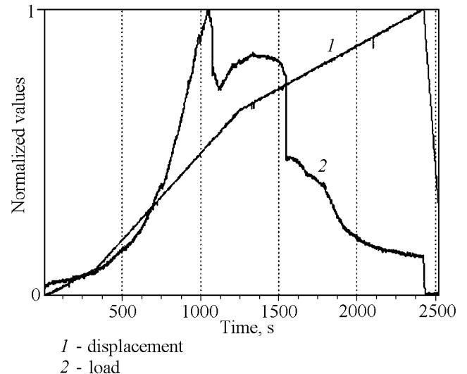
**Figure 1.** A demonstration sample loading curve with a supercritical load portion. Max. displacement = 3.09 mm, max. load = 5.361 t.
