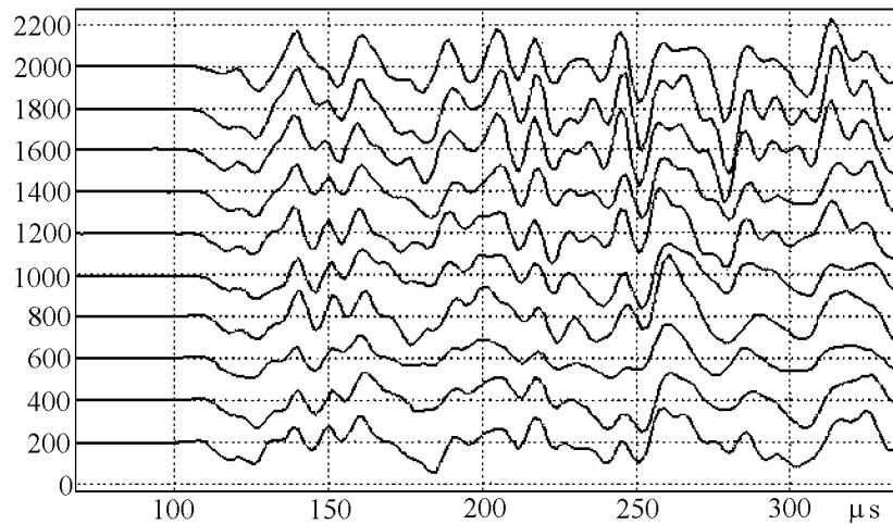
**Figure 7.** The wave pattern obtained on the metallic cylinder. Coordinate  $Z$  (direction is normal to the axis of the cylinder).
