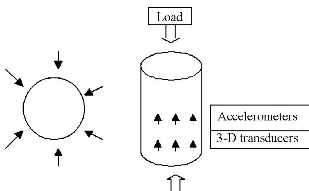
**Figure 3.** Arrangement of the recording transducers on the sample surface.
