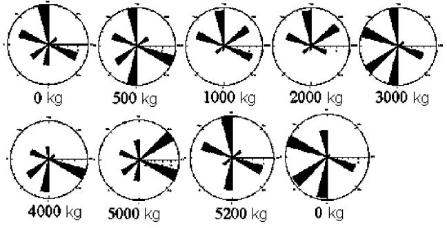
**Figure 10.** The azimuthal distribution of the supersonic wave velocity (data of the 3-D transducers). The moment of the wave arrival determined from the first half-cycle of the wave crossing the maximum. Symmetric routes.
