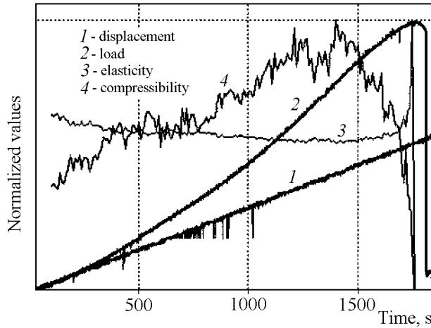
**Figure 4.** Loading curve (black) at a constant rate of deformation (blue). The corresponding elasticity factor (black broken line) and the volume dynamic compressibility index. Max. displacement = 1.52 mm, max. load = 4.52 t.
