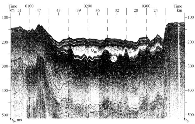
Figure 21. Example of seismic record of Cretaceous and Quaternary seismic units.
