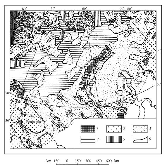
Figure 24. Magnitudes of neotectonic movements in the Barents-Kara region. 1 - 500 m; 2 - 500 to 0 m; 3 - 0 to -250 m; 4 - -250 to -500 m; 5 - < -500 m; 6 - isobases of recent movements.
