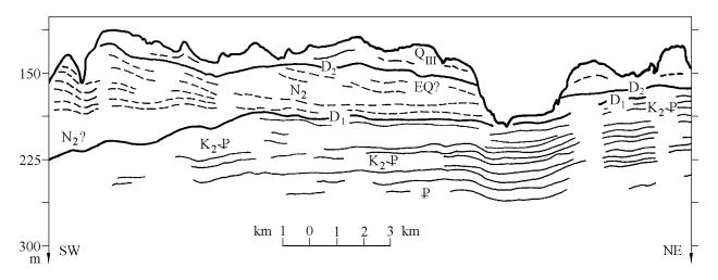
Figure 12. Interpretation of the record displayed in Figure 11 showing pre-Pliocene and recent erosional truncations.
