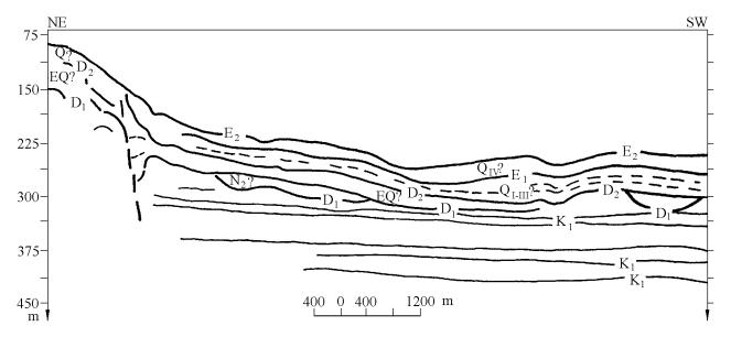
Figure 20. Interpretation of the record displayed in Figure 19 showing drape sheets of Quaternary seismic units.
