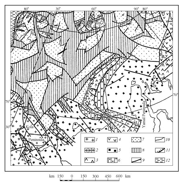
**Figure 23.** Neotectonic map of the Barents-Kara region. 1 – crystalline shields; 2 – graben-shaped troughs in crystalline shields; 3 – post-platform orogenic belts; 4 – outcrops of platform folded basement; 6 – pre-orogenic troughs; 7 – rises and knolls of continental-margin platform; 8 – trenches and troughs in continental-margin platform; 9 – active recent faults; 10 – plicated boundaries of newly formed structures; 11 – flexure-fault zone at the shelf edge; 12 – continental slope.
