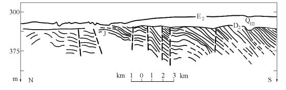
Figure 5. Interpretation of the record displayed in Figure 4 showing post-Jurassic faults and toplap at the Quaternary base.
