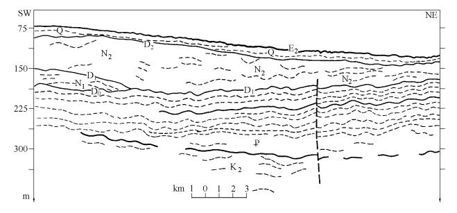
**Figure 14.** Interpretation of the seismic record displayed in Figure 13 showing the geometries of the tops and bottoms of the Paleogene, Miocene, Pliocene, and Quaternary sequences.
