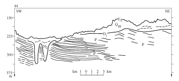
Figure 16. Interpretation of the seismic record displayed in Figure 15 showing Neogene erosion paleochannels.
