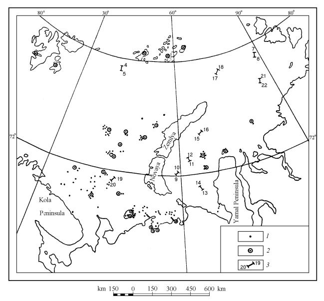
**Figure 2.** Location map of drill holes and fragments of reflection profiles. 1 – engineering-geological holes; 2 – stratigraphic wells; 3 – location of reflection profiles whose seismic sections are displayed in Figures 4–5 and 7–22.
